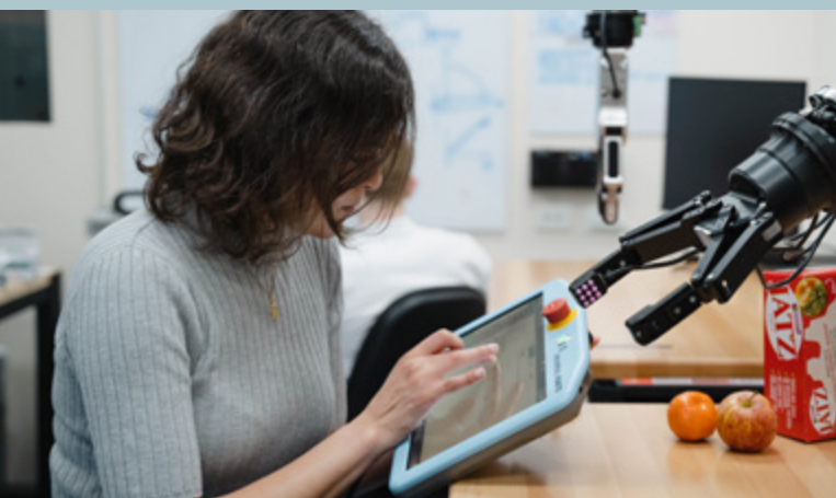
Co-founder Dr Heba Khamis, testing the prototype of Contactile's tactile sensor technology in a robotic gripping application.
